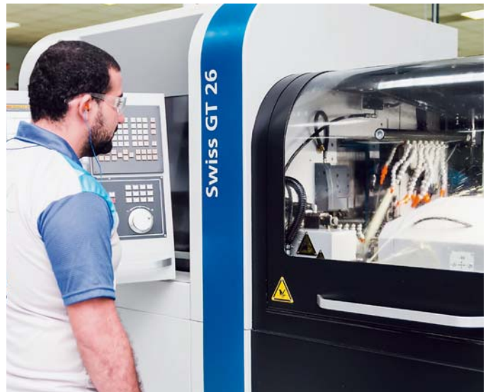
Mr. Leslie Bonilla, machine technician, in front of the Tornos Swiss GT 26, the machine is equipped with a gear hobbing device.
